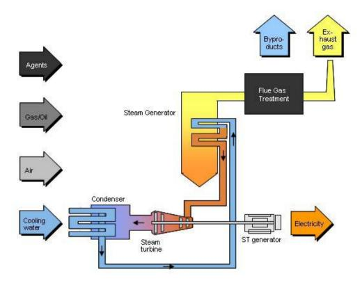
Steam power plant cycles are characterized by the pressure level at which they operate. Sub-critical cycles use pressures below the critical pressure of water. Typical popular unit sizes of large plants are in multiples of 125 /135 MW, 250/300 MW, 500 MW or 600 MW. On the other hand, supercritical cycles operate above the critical pressure providing higher efficiency. These cycles have varying unit sizes and varying parameters.
