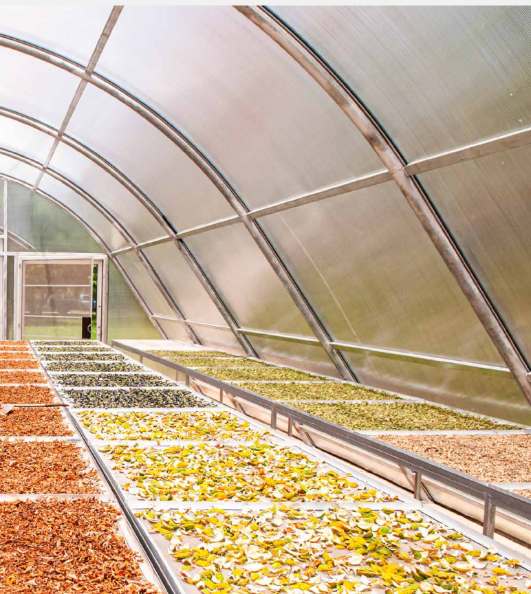
◀ Solar drying dome, Indonesia Used to dry agricultural and farm products by using the power of the sun to create heat.
